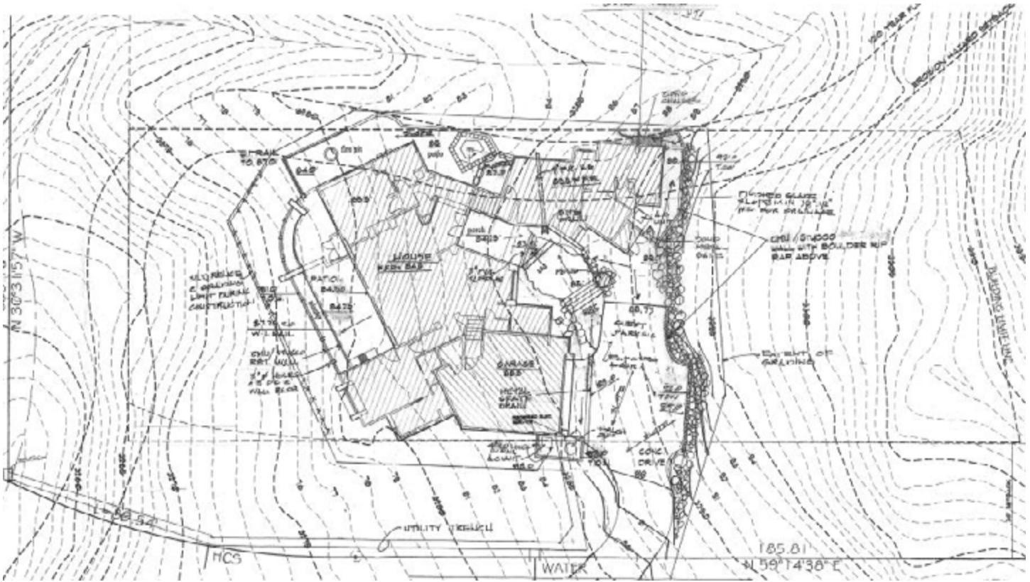
Image from a 2003 site plan that shows the potential for damage to a new building that met the minimum NFIP criteria. The building could still be impacted by channel erosion and local drainage.
